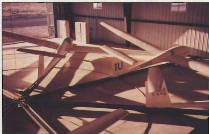
The carousel can accommodate gliders of greatly different sizes. Tow-out gear can be stored on the inboard ends of the beams.
