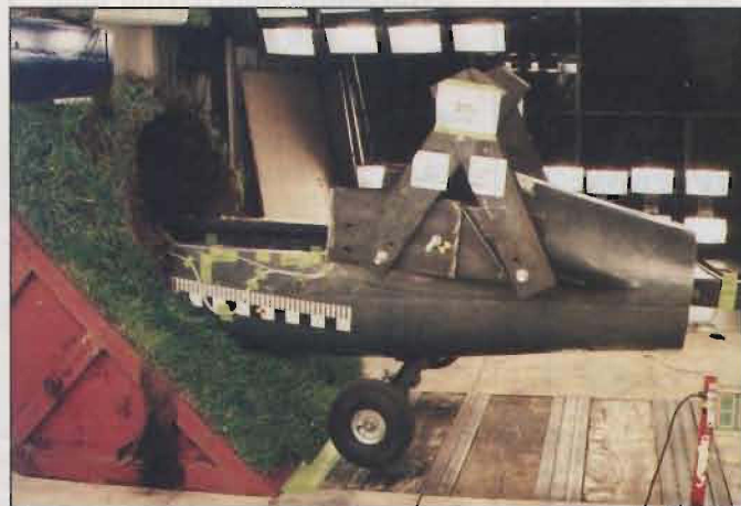
Figure 3: Martin Sperber's 'racing car cockpit' being tested at TÜV Rheinland in January 1998. Photo: Jochen Ewald.
